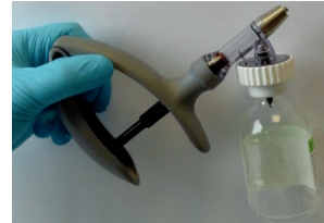
fig.3: Tighten the adapter to the syringe without turning the bottle itself.
