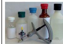
fig.2: Stick the spike central in the bottle, without turning the bottle itself.
