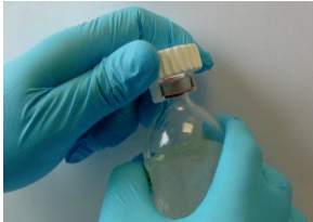
fig.1a: Select the corresponding adapter for the corresponding bottle. Introduce bottle in universal
