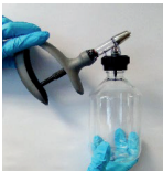
fig.1b: FOR THREADED BOTTLES ONLY: Hold the HSW ECO-MATIC® with the spike downwards and screw the threaded bottle into the adapter. Dismantling is carried out in the reverse order.
