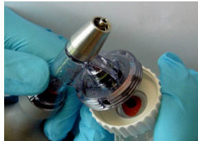
fig.2: Stick the spike central in the bottle, without turning the bottle itself.
