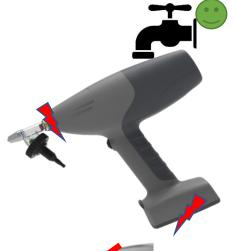
When cylinder is mounted and the battery slot is closed you can clean the device under running water.
