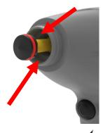
Please let the cylinder mounted for the cleaning, because without thecylinder, liquid could enter via the plunger opening and will destroy the electronic.
