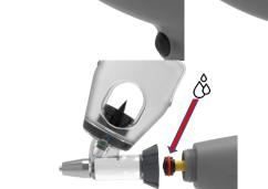
Lubricate the O-ring and then mount the new cylinder.
